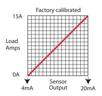
The C-1205 produces a loop-powered 4-20mA DC output proportional to monitored current up to 15 amps.
