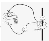
Remember to consider the ratio of the CT secondary to the sensor full-scale range to determine sensor output. Example: A 200:5A CT will produce 5 amps max, which is 1/3 of the 15 amp full-scale range of the C-1205. Applying this ratio (1/3) to the 16mA output range (20mA - 4mA) gives a 5.33mA signal change for a reading of 9.33mA at 200 A.
